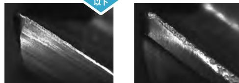
切削条件:  $n = 1,200 \text{ min}^{-1}$ ,  $V_f = 140 \text{ mm/min}$ ,  $a_p = 4 \text{ mm}$
